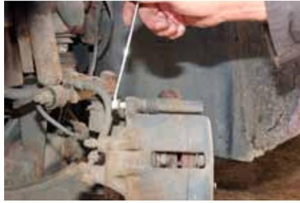
**2.** Undo the two 12mm slider bolts, then lever off the caliper and suspend it out of the way. Be very careful not to over stretch or strain the brake flexi-hose - support it so the weight does not hang on the hose.
