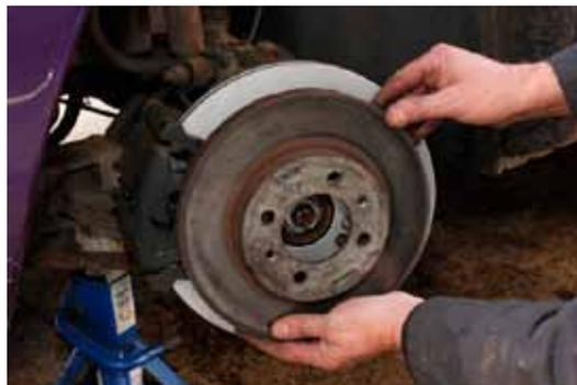
**Middle left:** New big disc kit from MGFMania is 280mm in diameter, making them 40mm larger than standard discs.
