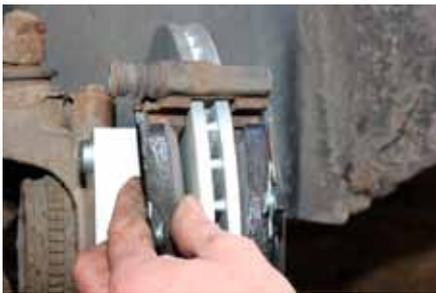
**10.** New brake pads must be fitted with the new discs - do not reuse the old brake pads. Apply a smear of copper grease to the top and bottom edges of the pads (not the braking surface) before fitting them.
