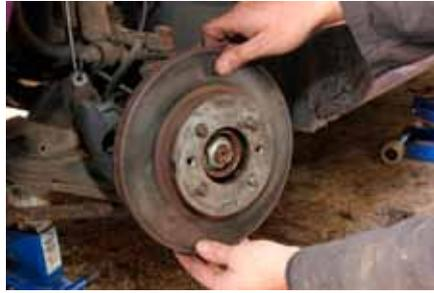
**5.** With any retaining screws removed, try to remove the brake disc. This can be difficult. If it's stuck, you should use a puller, even though many people resort to a lump hammer (wear goggles if you do).
