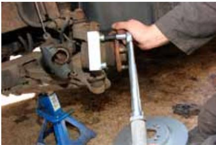
**7.** An anodised aluminium bracket needs to be fitted to make room for the larger discs. Two 10mm allen key headed bolts are supplied in the kit, which must be fitted with thread lock and tightened to 85Nm.
