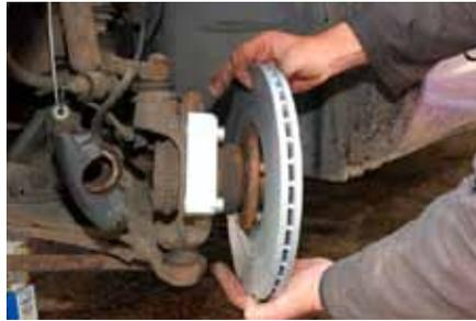
**8.** The new vented brake disc can now be fitted onto the hub. The original disc retaining screws are not required and the brake disc will remain secure once the wheel bolts have been fitted.
