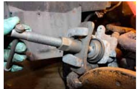
**12.** Fitting larger discs to the rear brakes is similar to the fronts. The only difference concerns retracting the caliper's piston, where a wind-back tool is required to turn the piston instead of pushing it in.
