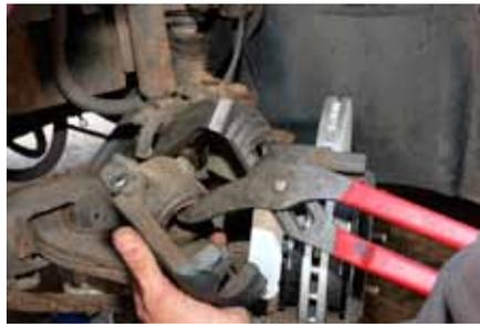
**11.** With new, thicker brake pads fitted, it may not be possible to refit the caliper, so retract its piston - you can carefully use a large pair of water pump pliers. Once refitted, hand tighten the two slider bolts.
