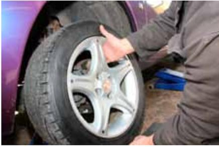
**1.** Raise a front corner of the vehicle using a trolley jack carefully positioned under the jacking point, lower it onto an axle stand underneath the front subframe, then remove the road wheel.
