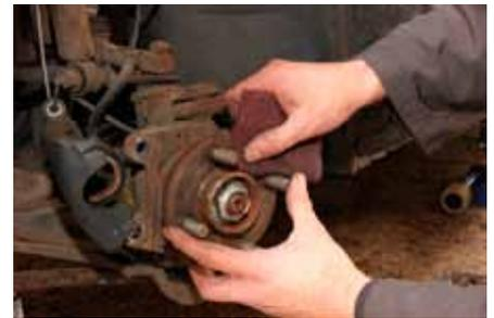
**6.** After removing the brake disc, clean the mating surface of the hub against which the old disc sat. This surface needs to be thoroughly clean to ensure the new disc sits flush and rotates true.
