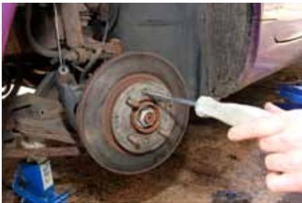
**4.** Undo any retaining screws for the brake disc. These can be seized, so hit them with a hammer and impact screwdriver to help shock and release them. They may need drilling out if they are damaged.
