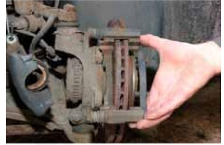
**3.** Remove the old brake pads, then undo the 15 or 16mm caliper carrier bolts. Be warned - these will be tight. Remove the caliper carrier, clean it thoroughly and check the slider bolts are free.
