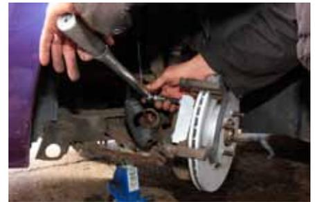
**9.** The caliper carrier can now be refitted and secured with new 10mm allen key bolts. Apply a smear of thread lock to them before fitting, then tighten them with a torque wrench to 85Nm.
